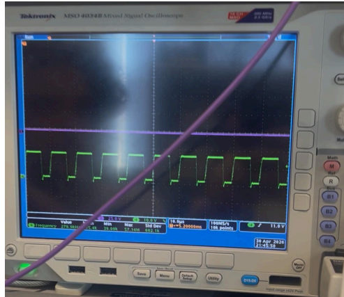
Figure 5: PWM square wave for boost converter
