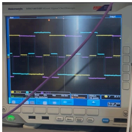
Figure 11: Final 3-Phase Output Waveforms
