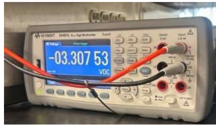
Figure 9: Probed voltage difference between ground and 3.3 V output of LDO
