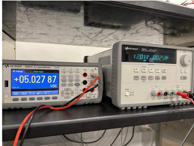
Figure 14: 12.01V Power Supply Input Being Bucked Down To 5V Using A Multimeter
