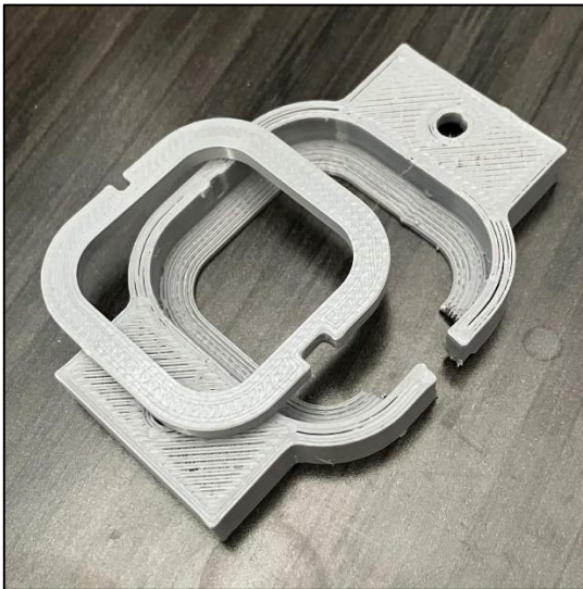
Figure 9 Augmented 3D print of the Load Cell (area for wires to pass though was expanded)
