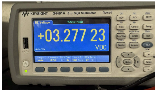
Figure 16: 3.3 V buck output
