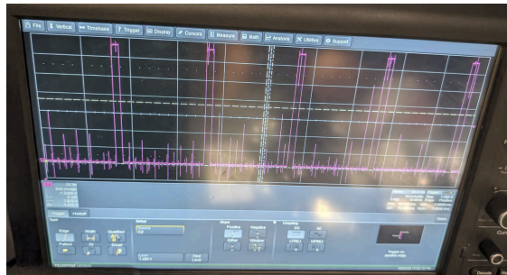
Figure 27: Driver PWM Signal on Oscilloscope
