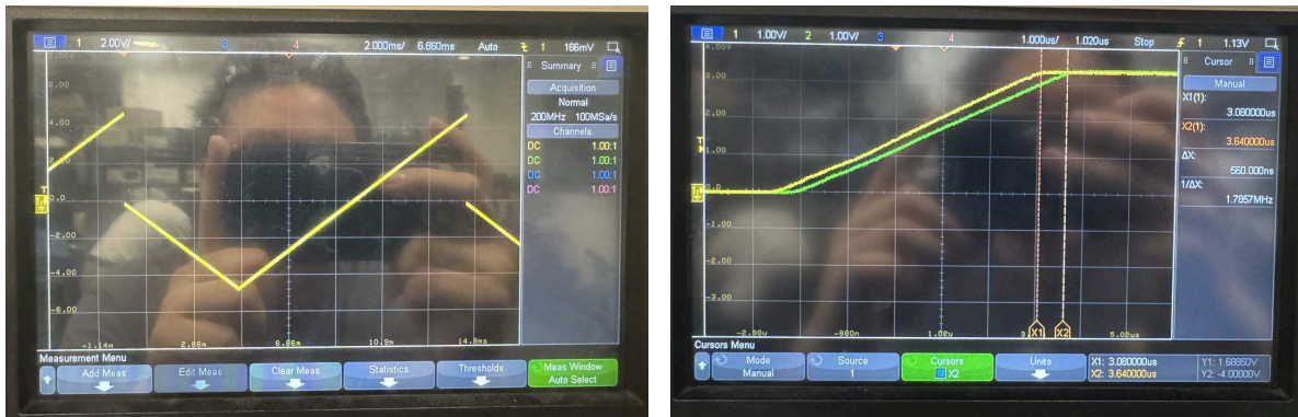
Figure 13: Oscilloscope measurements of the DAC code sweep showing smooth increasing output behavior (left) and RAW_X/RAW_Y update timing with a 560 ns delay between channels (right)
