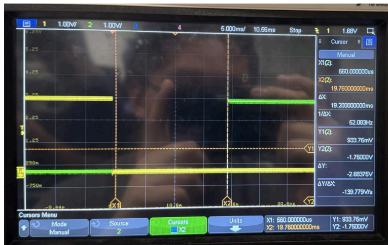
Figure 12: Oscilloscope measurement of user input latency, showing the delay between the input event and system response
