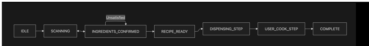
Figure 7: Backend state machine for scanning, recipe generation, dispensing, and completion.
