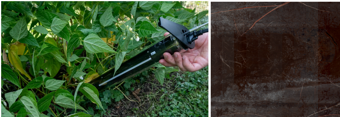
Figure 2a (left): Example of field operation of CI-60X Series root imaging system Figure 2b (right): Example output image for CI
