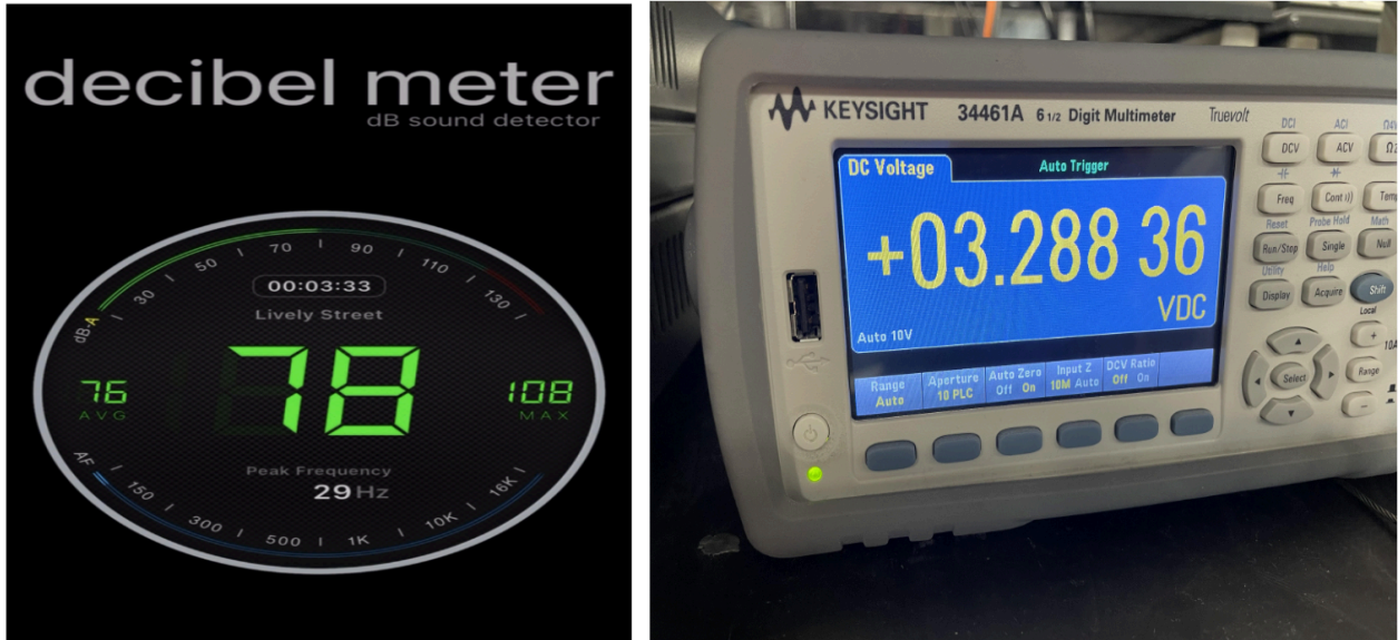
Figure 14. Alarm Subsystem Sound and Voltage Measurements
