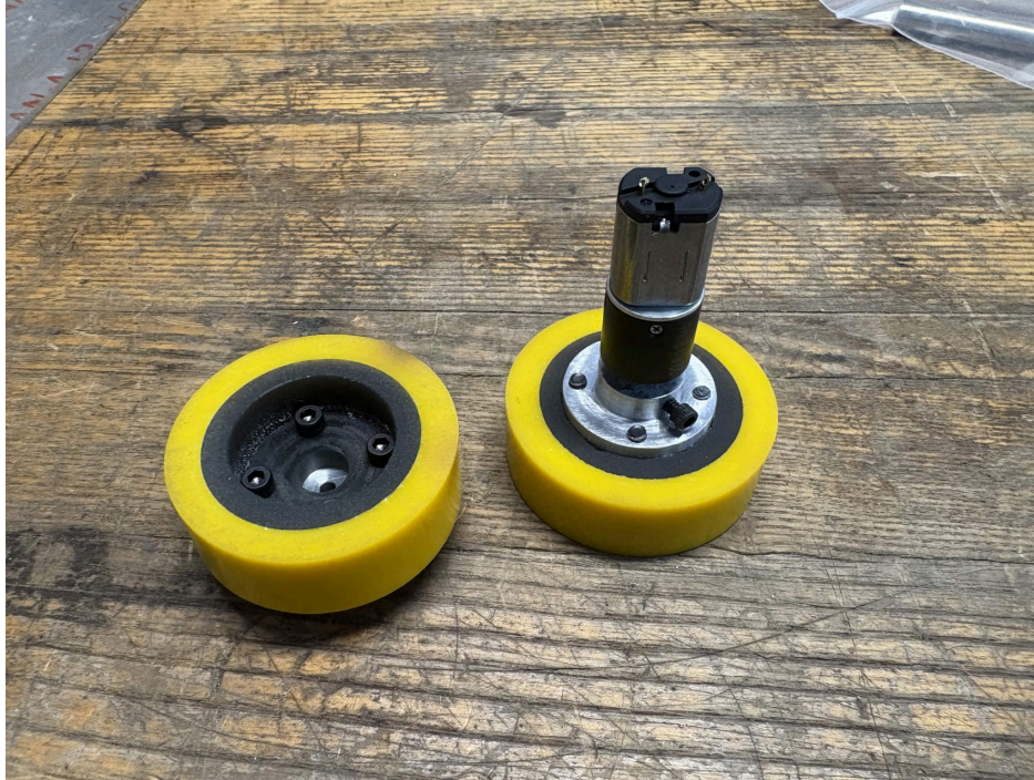
Figure 2: The polyurethane wheel + metal wheelhub + gearmotor assembly is depicted.
