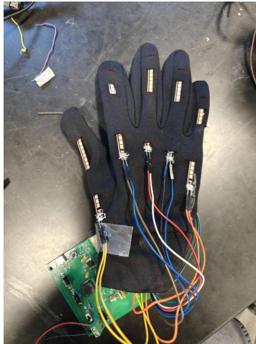
Figure 3 Flex Sensor Glove. Each of the four fingers has a flex sensor connected to it while the thumb has two (one above and one underneath). The flex sensors are attached to the PCB via 2x1 conn pins.
