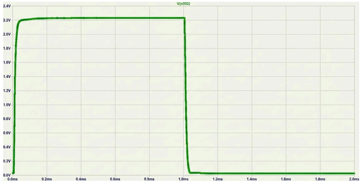
Figure C4: Step response of simulated circuit for 5 \mu A pulse. No overshoot, and settling time of 73 \mu s
