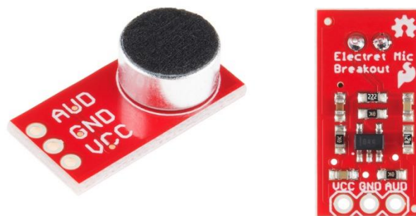
Fig 3. Sparkfun Electret Microphone with preamp [1].
