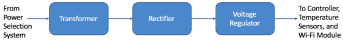
Figure 13. AC/DC Converter Block Diagram
