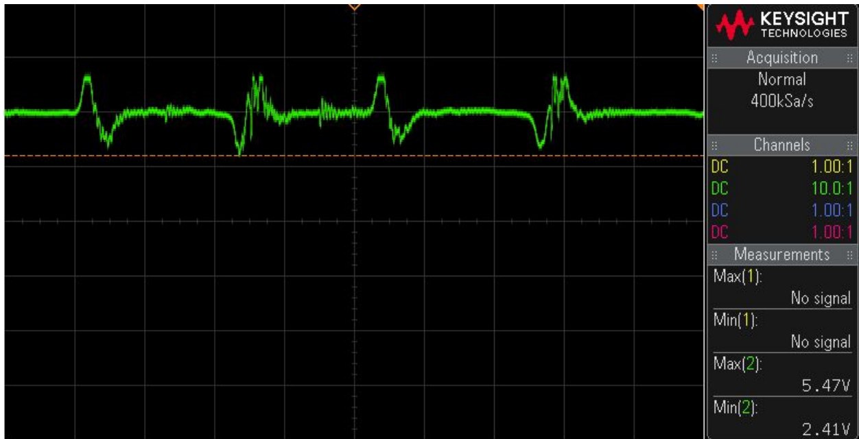
Figure 2.6: Accelerometer Output Waveform
