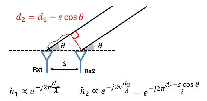
$\Delta \Phi = \angle h_2 - \angle h_1 = 2\pi s \cos \theta / \lambda \mod 2\pi$
