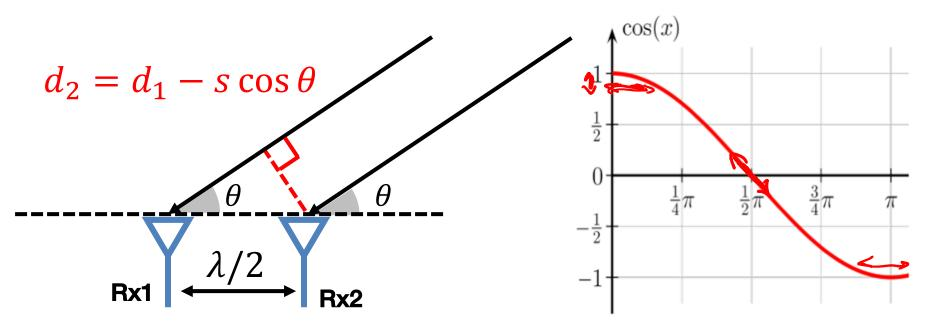
Pros: More accurate than RSSI, Simple! Cons: Ambiguity:  $\cos \theta = \cos(-\theta)$ Error not linear with  $\theta$  due to  $\cos \theta$ Does not work with multipath!
