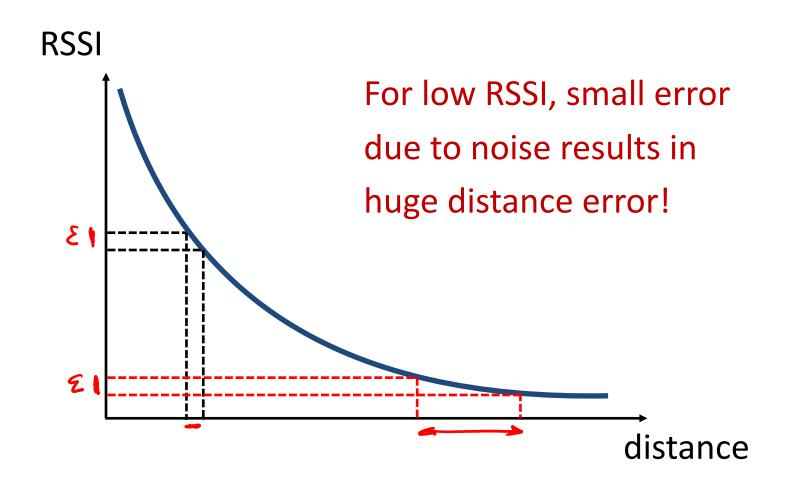
Method 1: RSSI Based Localization **Pros:** Very simple, no hardware modifications! **Cons:** Highly inaccurate! Does not work with multipath! **RSSI**  $h \propto \frac{1}{d_1} e^{-j2\pi \frac{d_1}{\lambda}} + \frac{1}{d_2} e^{-j2\pi \frac{d_2}{\lambda}}$  $RSSI \propto |h|^2 \neg \frac{1}{(d_1)^2} \text{ or } \frac{1}{(d_2)^2}$ Λ stance
