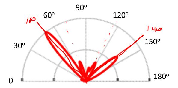
Method 3: Antenna Arrays (ArrayTrack Paper) Which is the Line-of-Sight Path (Direct Path)? Strongest Path!
