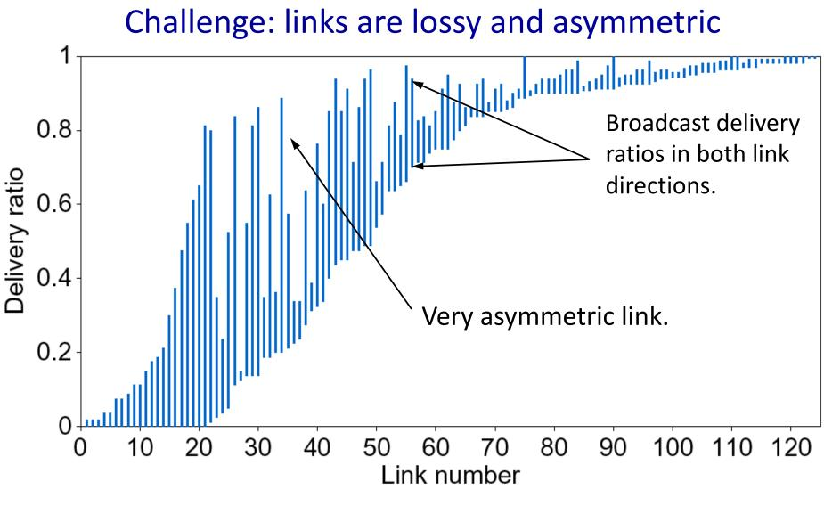
Different links have different loss rates Further, the loss rate may be different in each direction
