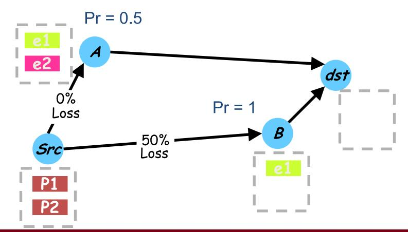
Compute forwarding probabilities without coordination using loss rates
