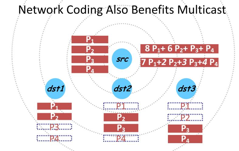
Without coding  $\rightarrow$  source has to retransmit all 4 packets With network coding  $\rightarrow$  2 packets are sufficient
