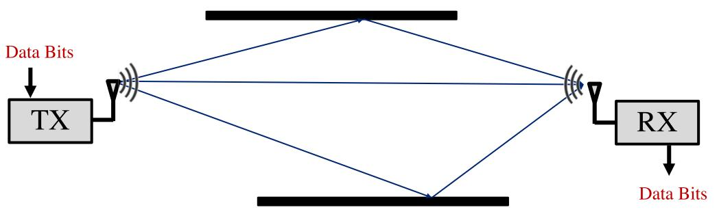
*Multipath Propagation:* radio signal reflects off objects ground, arriving at destination at slightly different times
