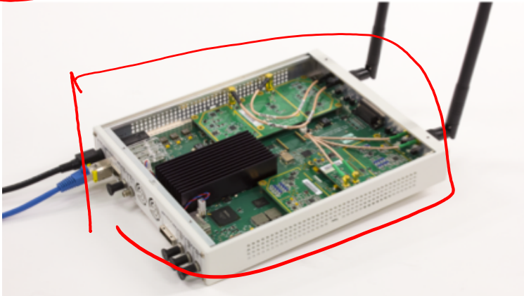
USRP : Universal Software Radio Peripheral (Ettus)
