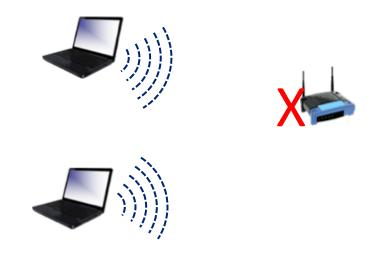
interference from other sources: standardized wireless network frequencies (e.g., 2.4 GHz) shared by other devices (e.g., phone); devices (motors, microwaves, baby monitors, ... ) interfere as well
