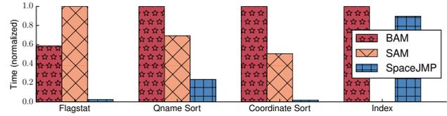
Figure 11: SAMTools vs. an implementation with SpaceJMP. BAM and SAM are alternative in-memory serialization methods; SpaceJMP has no serialization.
