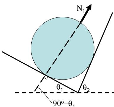
The normal force is always directed perpendicular (i.e. "normal") to the surface that provides it. If we extend  $N_1$ 's direction back to the surface that provides it, we meet that surface at a right angle, as shown.
