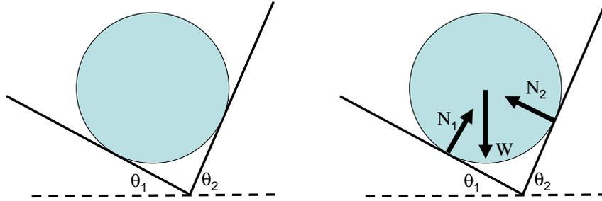
We know that the sphere is resting on the incline. We know the mass of the ball, as well. We are also assumed to know the two angles of the incline,  $\theta_1$  and  $\theta_2$ . We know that there is a gravitational force (the weight) pulling the sphere straight down. Therefore, there must also be a normal force on the ball from each plane to keep the ball from penetrating the surfaces.
