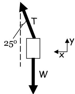
The relationship between forces and acceleration is given by Newton's Second Law,  $\vec{F}_{\text{net}} = m\vec{a}$ . To find the net force, we'll need to know the directions of all the forces in the problem. We know the weight points straight down (all y-direction), and the tension in the string has a positive x-component and a positive y-component (i.e. "up and to the left").
