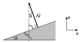
The angle marked with a double arc has the value  $90^{\circ}$ - $\theta$ . The Normal force therefore makes an angle of  $\theta$  with the y-axis (i.e. the vertical).
