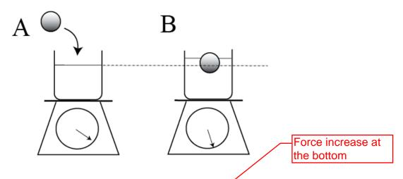
8. How much larger is the pressure at the bottom of the container in B than in A?
