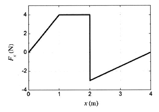
2) A force is exerted on an object along the x-axis as shown above. What is W, the work done by the force on the object during the displacement from 0 to 4 m?
