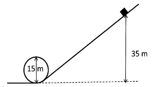
A block of mass  $50 \ kg$  is about to roll down a roller coaster track as shown above. Its initial height is  $35 \ m$  and the diameter of the circular loop is  $15 \ m$ . Assume that friction and air resistance are negligible.
