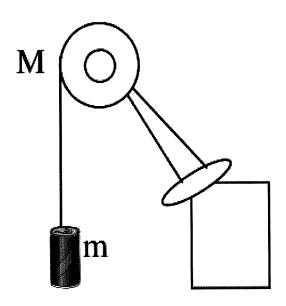
A uniform disk of unknown mass M and radius R=10~cm is free to rotate around a fixed horizontal axle supported in frictionless bearing. A light string is wrapped around the rim of the disk and then tied to a mass  $m=60\ g$  . The string does not slip as it unwinds on the disk. When released the mass moves down with acceleration 3.27  $m/s^2$  . Take  $g=9.8\ m/s^2$  . The moment of inertia of a uniform disk is  $1/2MR^2$
