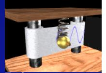
A 3 kg mass is attached to a spring (k=24 N/m). It is stretched 5 cm. At time t=0 it is released and oscillates.
