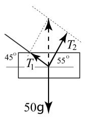
$$\begin{aligned} \boldsymbol{T}_1 &= (-T_1 \cos 45^\circ, T_1 \sin 45^\circ), \\ \boldsymbol{T}_2 &= (T_2 \cos 55^\circ, T_2 \sin 55^\circ), \\ \boldsymbol{F} &= (0, -50g). \end{aligned}$$
