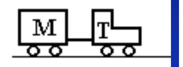
A tractor T (m=300Kg) is pulling a trailer M (m=400Kg). It starts from rest and pulls with constant force such that there is a positive acceleration of 1.5 m/s<sup>2</sup>. Calculate the pulling force of the tractor.
