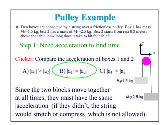
Big Idea: Apply N#2 to each block to first find acceleration, then use kinematics to find t.
