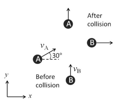
Two billiard balls, A and B, are moving on a frictionless table as shown above. Their masses are  $m_A = 0.8$  kg and  $m_B = 0.5$  kg. Before collision, ball A is moving in the direction  $30^\circ$  off the x-axis with speed  $v_A = 6$  m/s, while ball B is moving along the +y-axis with speed  $v_B = 2$  m/s. After collision, ball A moves along the +y-axis, while ball B moves along the +x-axis. Ignore air resistance.
