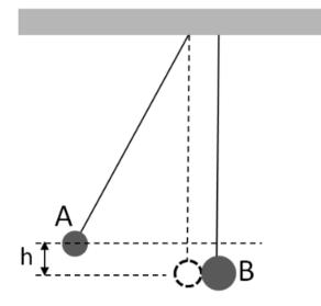
Two pendulum bobs made of soft clay hang from a ceiling as shown above. The mass of bob A is  $m_A = 1 \ kg$  and that of bob B is  $m_B = 2 \ kg$ . Initially, the height of bob A is h and bob B is at rest. They stick together after collision.
