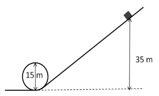
A block of mass 50 kg is about to roll down a roller coaster track as shown above. Its initial height is 35 m and the diameter of the circular loop is 15 m. Assume that friction and air resistance are negligible.
