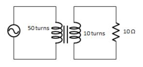
16) What is the average power dissipated in the resistor?
