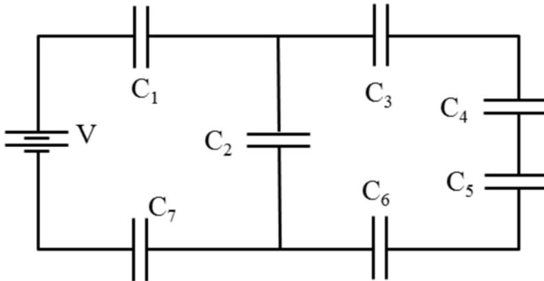
Seven identical capacitors with capacitance  $C = 8.5 \text{ nF}$  are connected to a 12 Volt battery as shown in the figure above.
