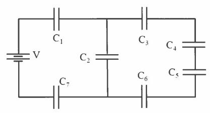
Seven identical capacitors with capacitance C = 8.5 nF are connected to a 12 Volt battery as shown in the figure above.
