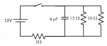
25. What is the current through the 5  $\Omega$  resistor immediately after the switch is closed?
