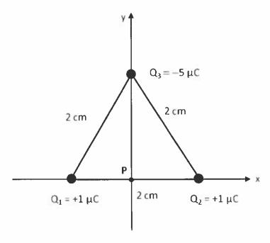
11. How much work W is required by you to assemble the three charges to this configuration?
