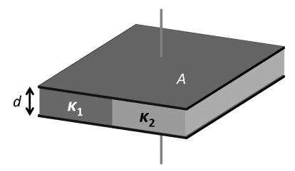
Calculate the capacitance C of this capacitor.
