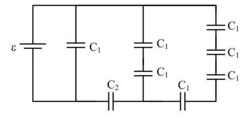
23. What is the equivalent capacitance of the circuit diagram above if all the capacitors have capacitance C?
