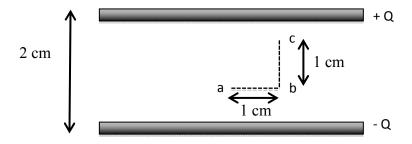
11. How much work  $W_{ab}$  would you have to do to move a +1.0 C charge horizontally by 1 cm from point  $\underline{\bf a}$  to point  $\underline{\bf b}$ ? How much work  $W_{bc}$  would you have to do to move a +1.0 C charge vertically by 1 cm from point  $\underline{\bf b}$  to point  $\underline{\bf c}$ ?
