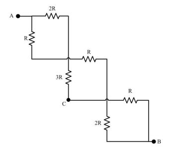
19. What is the equivalent resistance of the circuit elements between points A and B in terms of resistance R?
