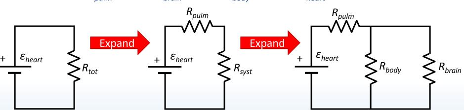
$$R_{pulm} = 12 \ \Omega, R_{brain} = 1 \ k\Omega, R_{body} = 160 \ \Omega, \varepsilon_{heart} = 120 \ V$$
