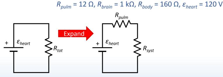
$R_{pulm}$  &  $R_{syst}$  are in series  $R_{tot} = R_{pulm} + R_{syst}$  $V_{tot} = V_{pulm} + V_{syst} = \varepsilon_{heart}$
