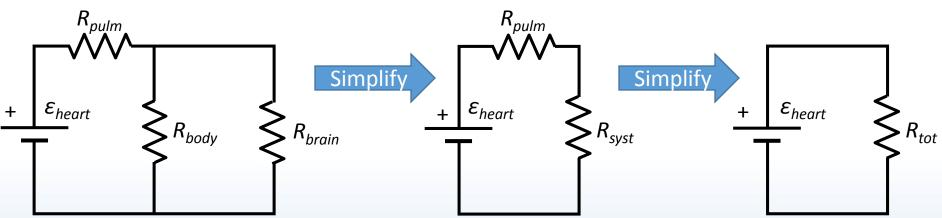
R<sub>brain</sub> & R<sub>body</sub> are in parallel  $\frac{1}{R_{syst}} = \frac{1}{R_{brain}} + \frac{1}{R_{body}}$  $V_{syst} = V_{brain} = V_{bodv}$  $I_{syst} = I_{brain} + I_{body}$
