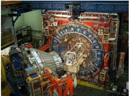
CDF Experiment. One of two Tevatron collider detectors. Now used for accelerator research
