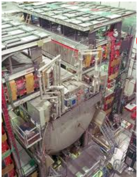
D0 Experiment. One of two Tevatron collider detectors, now used for liquid Argon R&D
