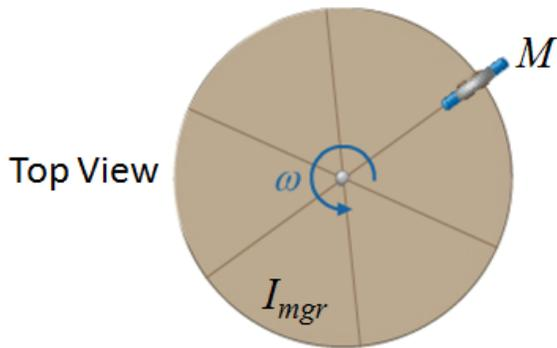
A child of mass  $M = 40$  kg is standing next to a merry-go-round having moment of inertia  $I_{mgr} = 834$  kg-m<sup>2</sup> and radius  $R = 2.3$  m. The merry-go-round is initially rotating with angular speed  $\omega_0 = 6$  rad/s. The child now jumps onto the outer edge of the merry-go-round and starts to rotate with it. You can treat the child as a point mass.
