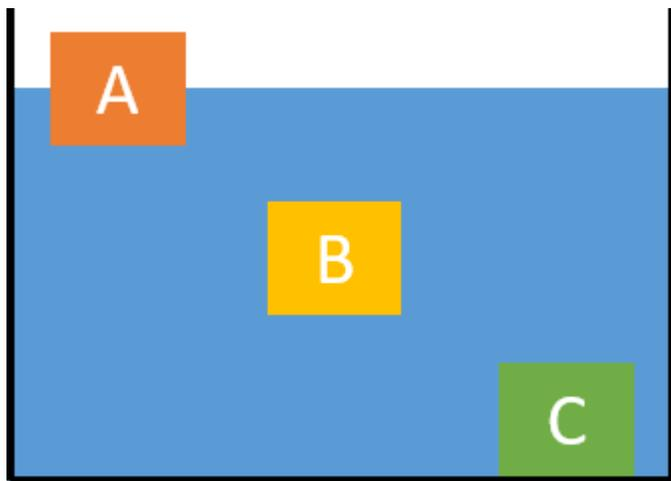
Three masses are in a swimming pool filled with water (density  $1000 \text{ kg/m}^3$ ). All three objects are identical in size ( $400 \text{ cm}^3$ ) but have different densities. Object A floats on the water (density  $580 \text{ kg/m}^3$ ), Object B is completely submerged underwater but has a density equal to that of water, and Object C sinks to the bottom (density  $3700 \text{ kg/m}^3$ ).
