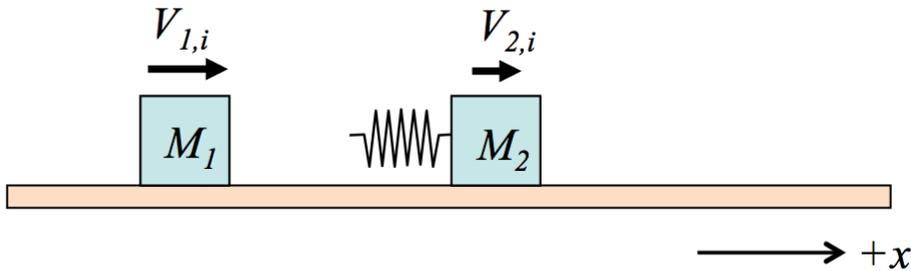
A block of mass  $M_1 = 2$  kg is moving to the right with initial speed  $V_{1,i} = 3.4$  m/s. It collides with another block of mass  $M_2 = 3$  kg that is initially moving to the right with  $V_{2,i} = 1.7$  m/s. There is a massless spring connected to the second block as shown, and the collision between the blocks is elastic. All motion is in one dimension and the  $+x$  direction is to the right in the picture.
