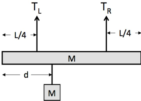
A beam of mass  $M=4.3$  kg and length  $L=5.1$  m is suspended by two vertical ropes as shown. The rope on the left has tension  $T_L$  and is attached a distance  $L/4$  from the left end of the beam. The rope on the right has tension  $T_R$  and is attached a distance  $L/4$  from the right end of the beam. A box that has the same mass  $M$  as the beam is suspended by a short rope which it attached a distance  $d$  from the left end of the beam.
