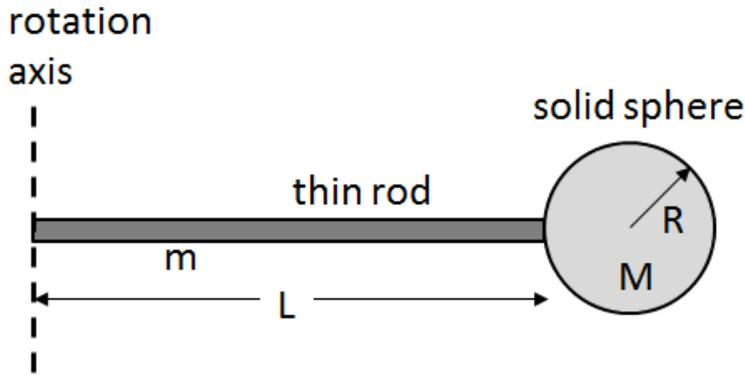
A uniform solid sphere having mass  $M$  and radius  $R$  is attached to the end of a uniform thin rod of length  $L$  and mass  $m$ . The moments of inertia of a rod and of a sphere are given in your formula sheet.
