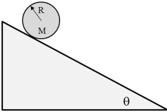
A hollow ball (spherical shell) having a mass  $M = 2.02$  and a radius of  $R = 0.171$  m is released from rest on a rough inclined plane which makes an angle  $\theta = 30^\circ$  with the horizontal. The static frictional force causes the ball to roll without slipping as it moves down the incline.
