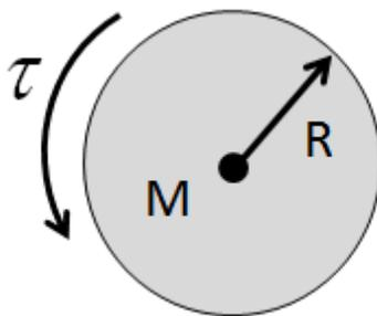
A uniform solid cylinder having mass  $M = 2.4 \text{ kg}$  and radius  $R = 0.43 \text{ m}$  is free to rotate around a fixed frictionless axle through its center (out of the page in the figure). The cylinder is initially at rest and at  $t = 0$  a constant torque with magnitude  $|\tau| = 9.763 \text{ Nm}$  is applied around the axis causing the cylinder to rotate.
