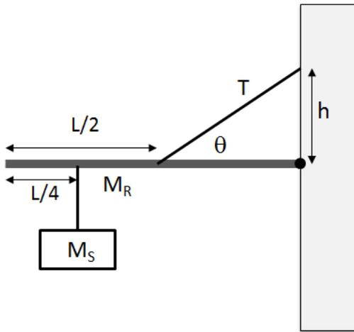
A horizontal rod of length  $L$  and mass  $M_R = 1.8 \text{ kg}$  is used to hang a sign on a wall. The right end of the rod is attached to the wall by a hinge. A wire having tension  $T$  runs from the center of the rod to a place on the wall a distance  $h$  above the hinge as shown. The wire makes an angle  $\theta = 28^\circ$  with the rod. The sign has mass  $M_S = 0.6 \text{ kg}$  and hangs distance  $L/4$  from the end of the rod. The system is in equilibrium.
