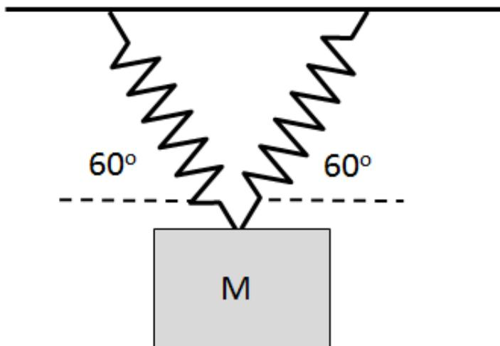
A mass,  $M = 3.2$  kg, hangs motionless from the ceiling from two identical ideal, massless, springs with spring constants  $k = 507$  N/M. Each spring makes an angle of  $\theta = 60^\circ$  with respect to horizontal as shown.
