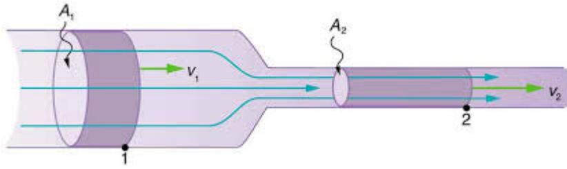
An incompressible fluid (density  $1000 \text{ kg/m}^3$ ) flows through a horizontal pipe with cross sectional area  $A_1 = 0.0045 \text{ m}^2$  and speed  $v_1 = 3.2 \text{ m/s}$ . The pipe tapers down to a cross sectional area of  $A_2 = 0.0019 \text{ m}^2$ .
