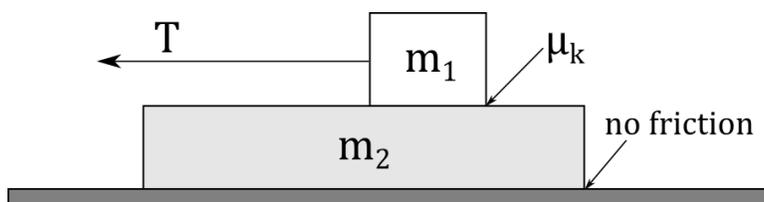
A box of mass  $m_1 = 2.1$  kg is being pulled by a horizontal string with tension  $T$  as shown. It moves to the left with a constant velocity across the top of a second box having a mass of  $m_2 = 5.1$  kg. The kinetic coefficient of friction between the upper box and the lower box is  $\mu_k = 0.6$ . There is no friction between the lower box and the horizontal floor, and the lower box accelerates to the left. Assume that the upper box is moving faster than the lower box.
