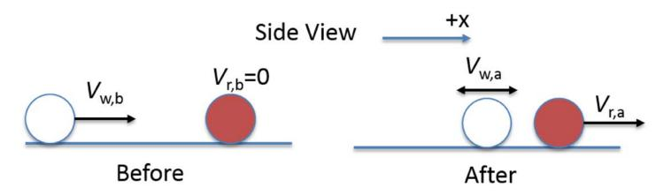
On a billiard table, a white ball strikes a red ball that was at rest before collision. After the collision, both balls are observed to move along the same line. The speed of the white ball before the collision is  $V_{\rm w,b} = 2$  m/s and after the collision is  $V_{\rm w,a} = 0.3$ . The speed of the red ball after collision is  $V_{\rm r,a} = 1.7$  m/s. The white and red balls have the same mass. (For this set of questions, assume the billiard balls are sliding on a frictionless surface).
