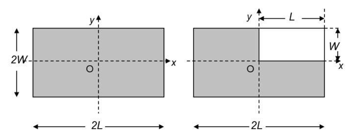
Consider a thin, uniform, solid, rectangular sheet of mass M, length 2L in the x-direction, and width 2W in the y-direction. It is placed symmetrically with respect to an (x, y)-coordinate system as shown in the left figure. Now, the upper right quadrant of this sheet is cut off, as shown in the right figure.
