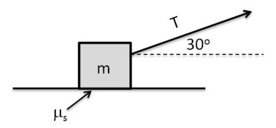
A block of mass m = 1.2 kg, at rest on a level surface, is being pulled by a string having tension T = 3 N at an angle of  $30^{\circ}$  above the horizontal, as shown in the diagram. Static friction keeps the block from moving. The coefficient of static friction between the block and the surface is  $\mu_S = 0.45$ .
