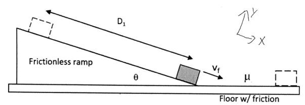
A 7 kg block starts at rest and slides down a frictionless ramp that makes an angle  $\theta$ =26 degrees with respect to the horizontal floor below. There is friction between the floor and the block. The length of the ramp is D<sub>1</sub> = 3 meters.
