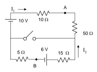
13. With the switch <u>open</u>, what is the current  $I_1$ ? (A positive sign means that current flows in the direction of the arrow.)
