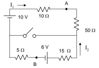
16. With the switch <u>closed</u>, what is the voltage difference,  $V_A$ - $V_B$ ?
