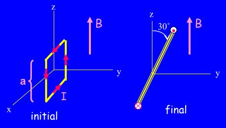
What is the direction of the magnetic moment of this current loop in its initial position?
