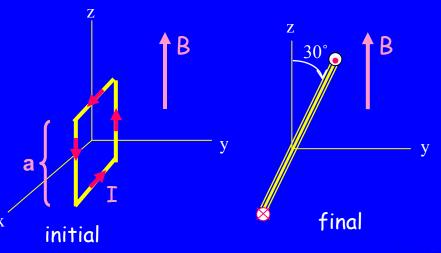
• What is the sign of the potential energy in the final state? (A)  $U_{\text{final}} < 0$  (B)  $U_{\text{final}} = 0$  (C)  $U_{\text{final}} > 0$
