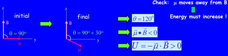
A square loop of side a lies in the x-z plane with current I as shown. The loop can rotate about x axis without friction. A uniform field B points along the +z axis. Assume a, I, and B are known.
