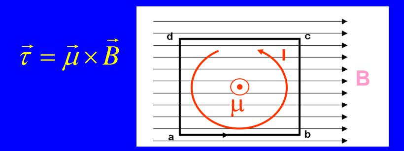
In this case  $\mu$  is out of the page (using right hand rule)
