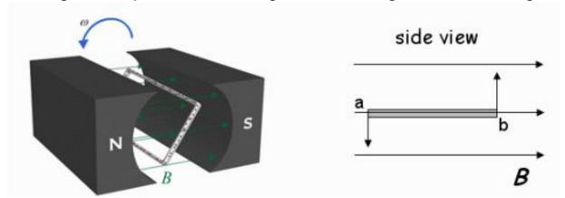
The side view of the loop is shown at a particular time during the rotation. At this time, what is the direction of the induced (positive) current in segment *ab*?
