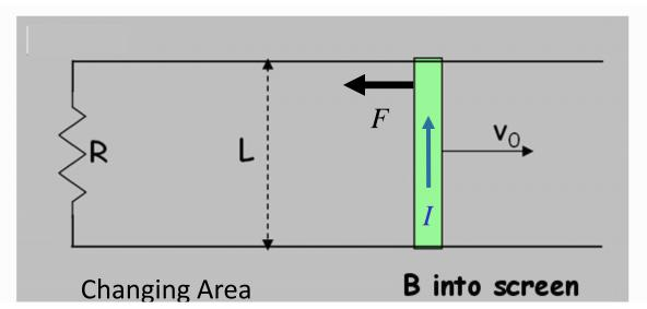
The entire apparatus is placed in a uniform magnetic field pointing into the screen, and the bar is given an initial velocity to the right.
