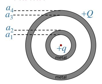
Point charge q at center of concentric conducting spherical shells of radii  $a_1$ ,  $a_2$ ,  $a_3$ , and  $a_4$ . The inner shell is uncharged, but the outer shell carries charge Q.
