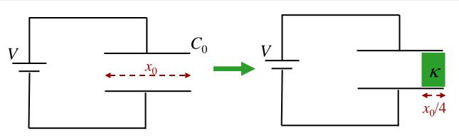
An air-gap capacitor, having capacitance  $C_0$  and width  $x_0$ is connected to a battery of voltage *V*.
