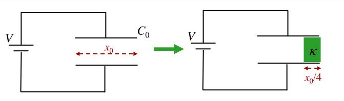
An air-gap capacitor, having capacitance  $C_0$  and width  $x_0$  is connected to a battery of voltage *V*.
