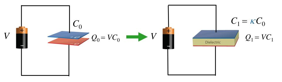
By adding a dielectric you are just making a new capacitor with larger capacitance (factor of  $\kappa$ )
