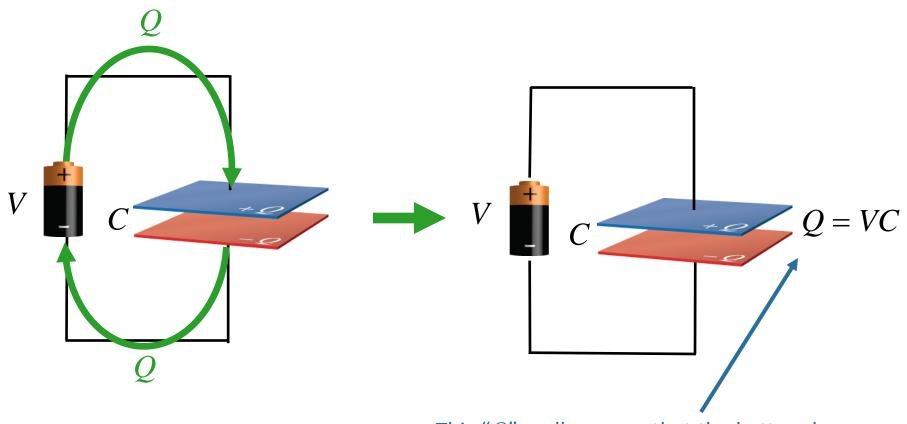
This "Q" really means that the battery has moved charge Q from one plate to the other, so that one plate holds +Q and the other -Q.
