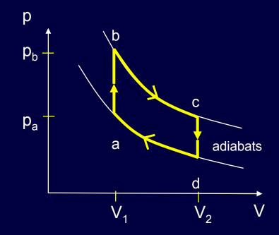
$$\varepsilon = 1 - \left(\frac{V_2}{V_1}\right)^{1-\gamma}$$
