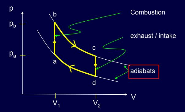
b→c and d→a are nearly adiabatic processes, because the pistons move too quickly for much heat to flow.
