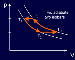
This refrigerator does not achieve Carnot efficiency, because both of the processes represented by the horizontal arrows involve irreversible heat flow between objects at different temperatures.
