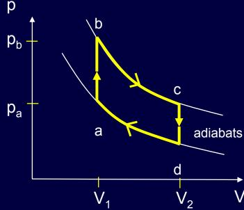
$$\begin{aligned} \mathbf{VV}_{by} &= \mathbf{VV}_{b \to c} - \mathbf{VV}_{d \to a} \\ W_{b \to c} &= U_b - U_c = C_v (T_b - T_c) \quad \text{because } \mathbf{Q}_{b \to c} = 0 \\ W_{d \to a} &= U_d - U_a = C_v (T_d - T_a) \quad \text{because } \mathbf{Q}_{d \to a} = 0 \\ W_{by} &= C_v (T_b - T_c) - C_v (T_a - T_d) \\ \mathcal{E} &= \frac{W_{by}}{Q_{in}} = \frac{C_v (T_b - T_c) - C_v (T_a - T_d)}{C_v (T_b - T_a)} = 1 - \frac{(T_c - T_d)}{(T_b - T_a)} \end{aligned}$$
