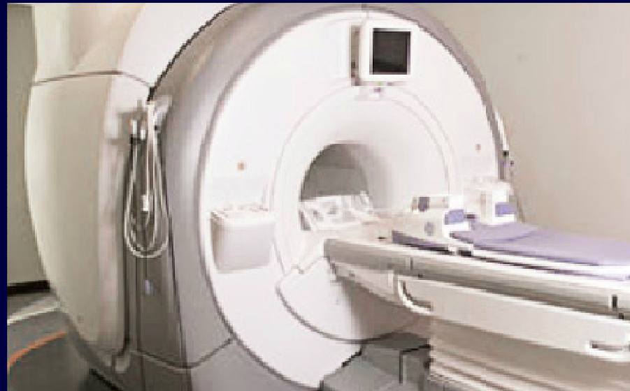
MRI's need liquid He to cool the superconducting magnets...
