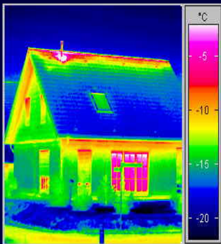
Heat loss through windows
